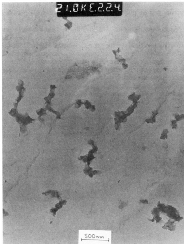
**Figure 1.** Transmission electron micrograph of a diluted, SDBS-stabilized polypyrrole colloid.
