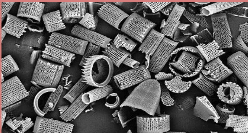
Figure 4: Diatomaceous Earth with one predominant type of Diatom [Micrograph courtesy of World Minerals]
