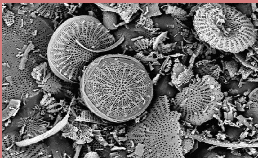
Figure 3: Diatomaceous Earth from freshwater deposit in Mexico [Micrograph courtesy of World Minerals]
