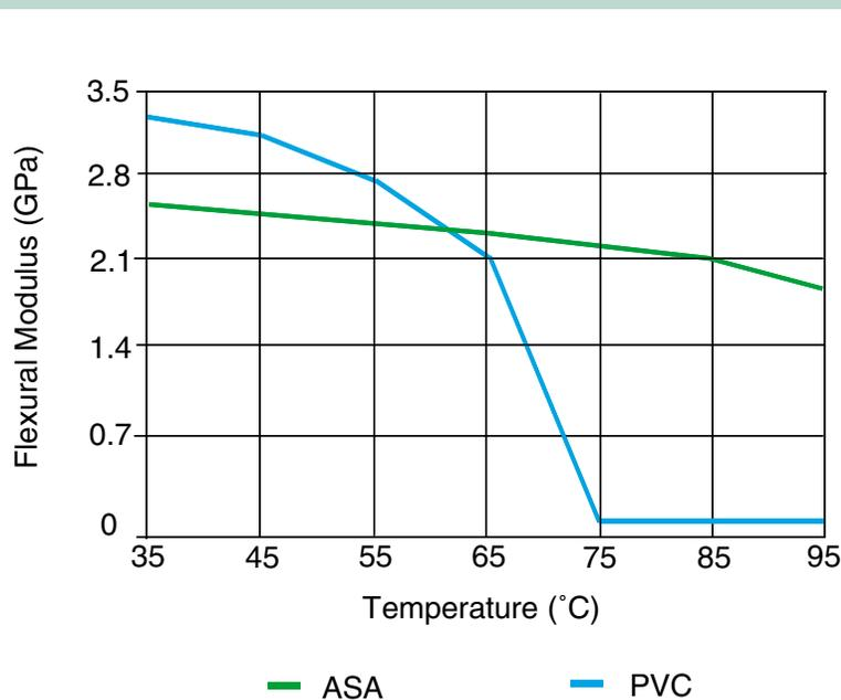
Figure 3: Stiffness of a standard ASA compared to rigid PVC at elevated temperatures.
