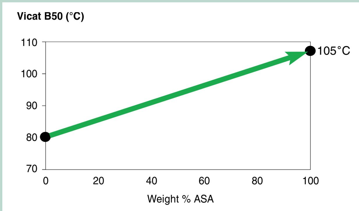
Figure 4: ASA increases the softening point of PVC.
