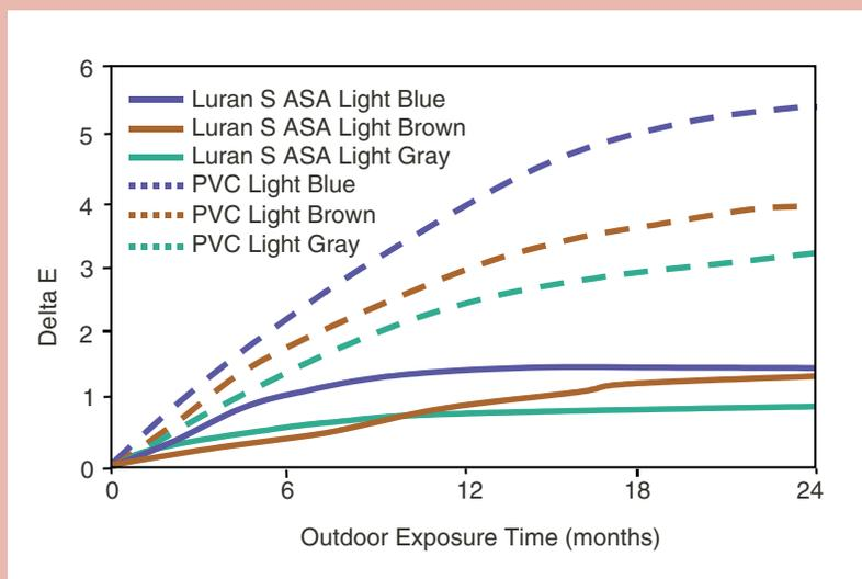
Figure 1: Outdoor ageing of PVC and ASA in Ohio, USA.
