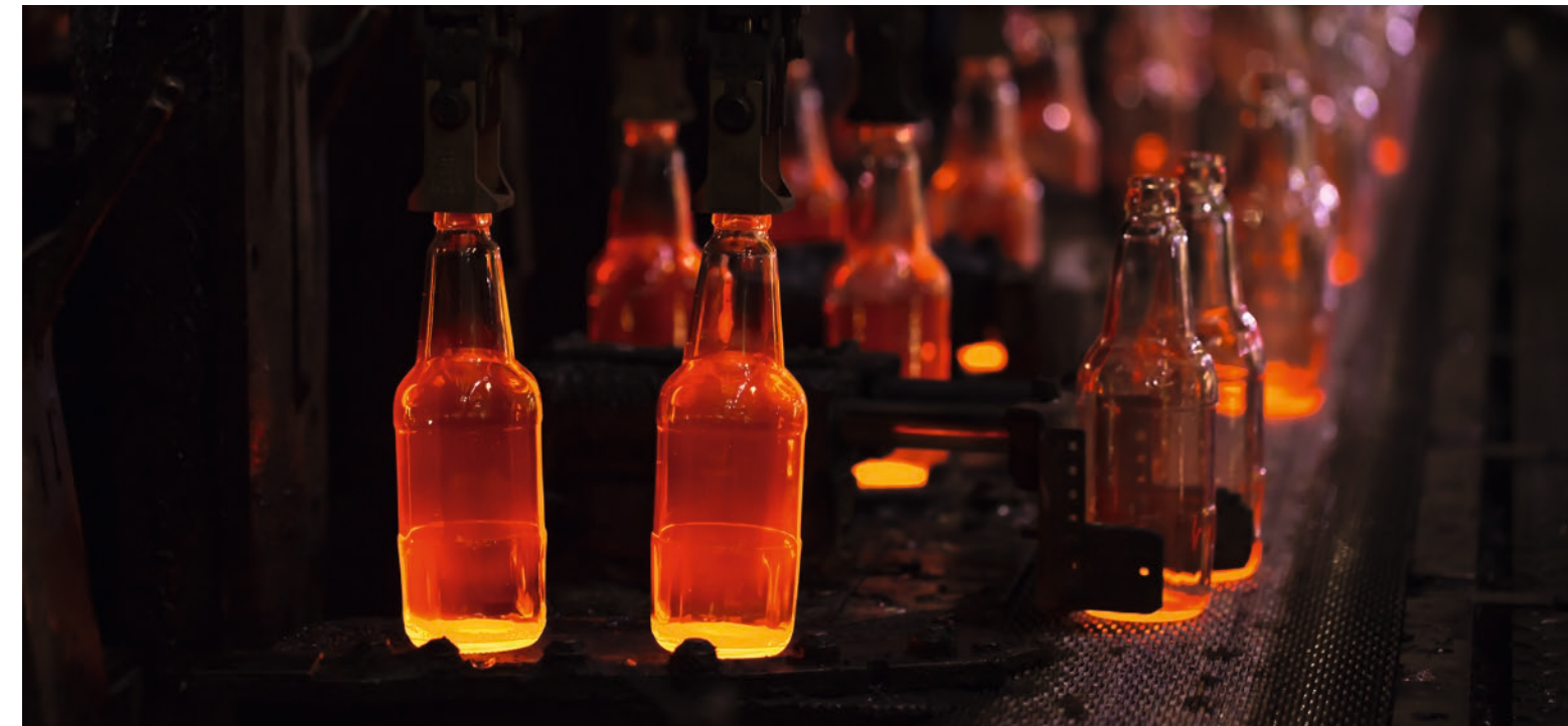
Molten glass is processed at ~1100°C (~2200°F), which is very energy intensive
