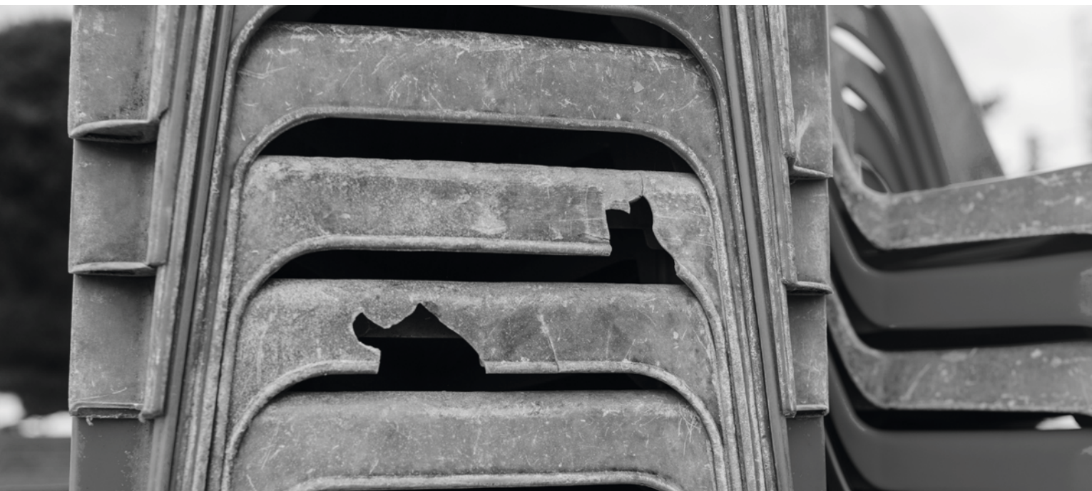
Polypropylene plastic garden chairs severely degraded by sunlight
